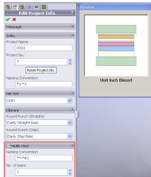
Swapping is possible in the die set process. Punches can be designed starting from parts or assembly. By all these, you may even divert layout process. Interference check can be saved for further use while with SolidWorks only it is visible but no saving and no further use.
